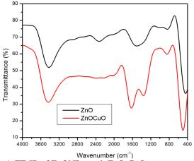
Fig. 4: FT-IR of ZnONPs, and ZnO-CuO, nanocomposites
